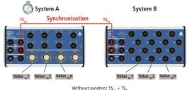
Without synchro:  $TS_{Ax} \neq TS_{B}$ , With synchro:  $TS_{Ay} = TS_{By}$
