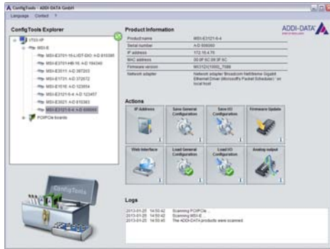
Example of monitor function: Testing the analog outputs – Value output without programming.
