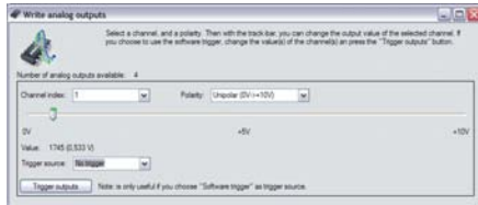
Example of monitor function: Testing the analog outputs – Value output without programming.
