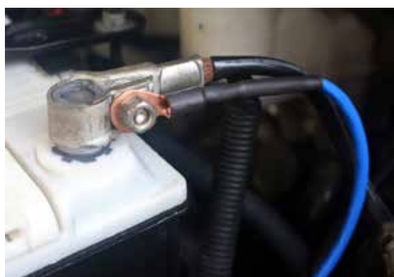
Typical Installation on Lead Acid Battery
