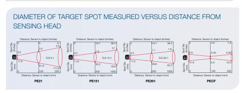
The PyroEpsilon Series is a range of high quality, low cost, compact sensors which measure the temperature of inaccessible or moving objects and materials. They measure temperatures from -20°C to 500°C, accurately and consistently, with an outstanding response time of 240 ms.
