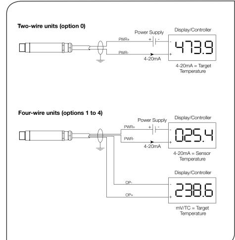
The PyroCouple Series is a range of high quality, low cost, compact sensors which measure the temperature of inaccessible or moving objects and materials. They measure temperatures from -20°C to 500°C, accurately and consistently, with an outstanding response time of 240 ms.
