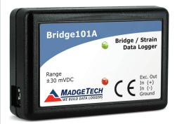
The Bridge101A Data Logger measures and records voltage, typically used in conjunction with strain gauges, load cells or other low-level DC voltage sources. This device is designed to accurately measure and record the output of the gauge to determine parameter levels such as stress, torque, strain, and pressure on a structure or item over a period of time.
