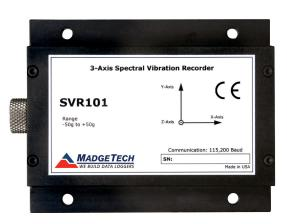
SVR101 only takes data when the *(user preset)* trigger level is exceeded. The minimum sampling rate is 2 seconds and the device can display peak X, Y and Z shock data, vector sum for data evaluated, up to 4 hours.
