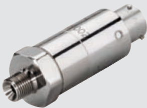
PHE220 Compact transducer for the harshest environments Very robust design for reliable measurements Built in electronics (0-5V or 1-6V) Operating temperature - 40°C /+125°C High accuracy from -1 bar up to +600 bar
