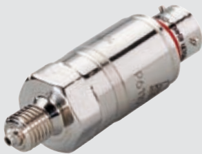
PHE160 Miniature transducer with built in electronics Available from 2 bar up to 600 bar Operating temperature -40°C to +140°C 0.5-4.5V DC with 8-30V DC power supply
