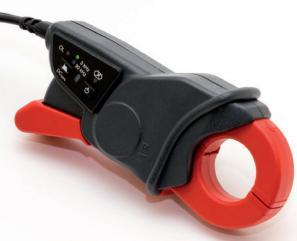
The quick, practical MH60 probe can be used for wide-band AC and DC current measurements thanks to its dual Hall effect / transformer technology. The MH60 probe can be powered either via its µUSB port connected to an oscilloscope, via a mains adapter or via its internal rechargeable battery combined with an automatic standby function which can be deactivated.
